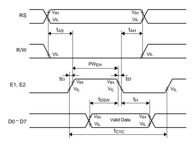
Fig.1 Bus Write Operation Sequence
